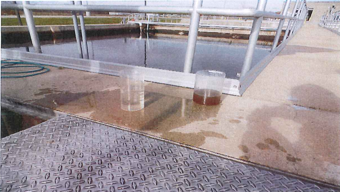
SBR 1 Clear Sample West Decanter and Dirty Sample East Decanter First 30 Sec.
